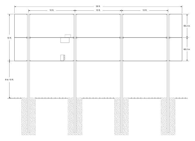
Once you have verified the positions of the posts and the size of the footings, you are ready to dig your holes, pour your concrete, and set your posts. There are several techniques for ensuring proper alignment of the posts. Typically installers will construct a temporary wooden support frame to hold each post in place while the concrete sets. Having plumb posts in the proper position is the key to a smooth mechanical installation.
